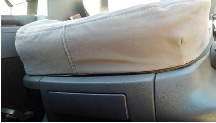
Photo shows elasticized edge located correctly in the indent at the bottom of the seat cushion.
